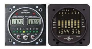
El's US-8 Ultimate Scanner displays absolute digital EGT information, as does JPl's EDM-700, and subsequent generations of digital engine monitors have all done the same.
